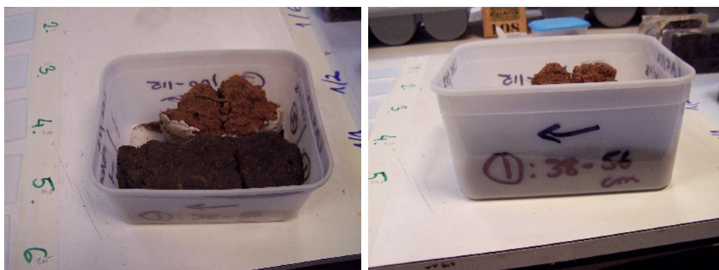
Figure 2: Blocks are put into labeled plastic containers ready for oven drying
