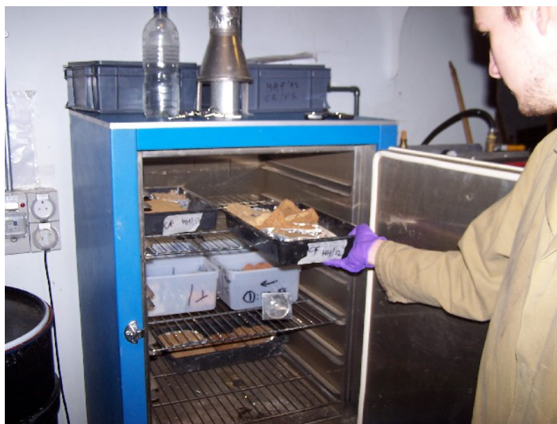
Figure 4: Placing samples in the oven for final drying
