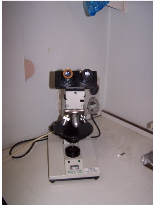
Figure 24: Check thickness of finished slides under the polarizer. Hand finish if required.
