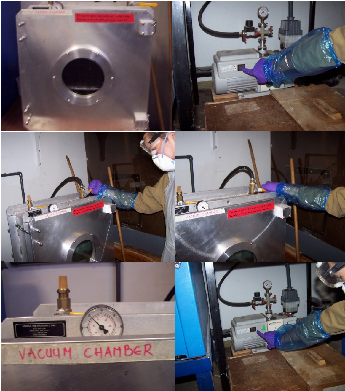
Figure 7: Increasing pressure in the vacuum chamber (l-r) close door, engage pressure by pulling lever down, turn on vacuum pump, wait for pressure to reach required, turn off pump
