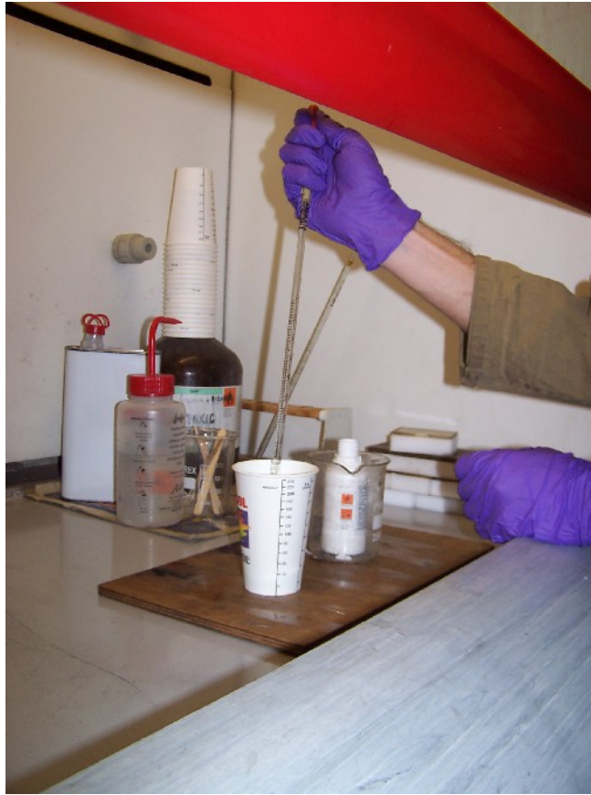
Figure 21: Add 0.7ml MEKP and stir until resin has changed from green to blue
