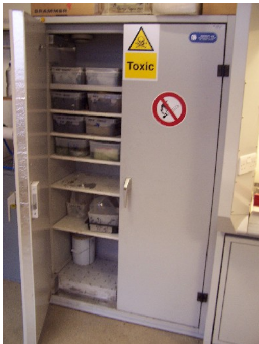
Figure 8: Curing cabinet with samples in storage
