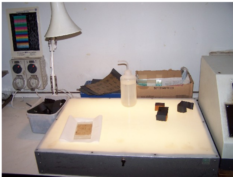
Figure 25: Hand finishing of slides on the light block using sand paper and oil.
