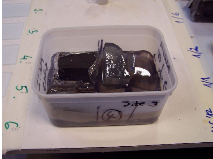
Figure 10: An impregnated block ready for sawing
