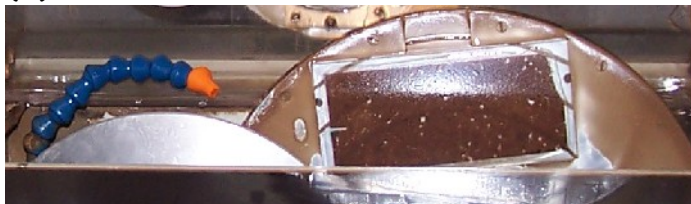
Figure 17: Sequence of beginning grinding after loading slides. 1: turn the machine from hand to auto. 2: turn on lubrication, and adjust nozzle accordingly (a). Wind grinding wheel two turns away from the slides (fig. 15), against the arrow direction. Set appropriate measurement to grind (fig. 15, 2) and set the gear (15.3). Close lid of machine. 3: start grinding wheel. 4: start sample holder, and flick gear on (15.4).
