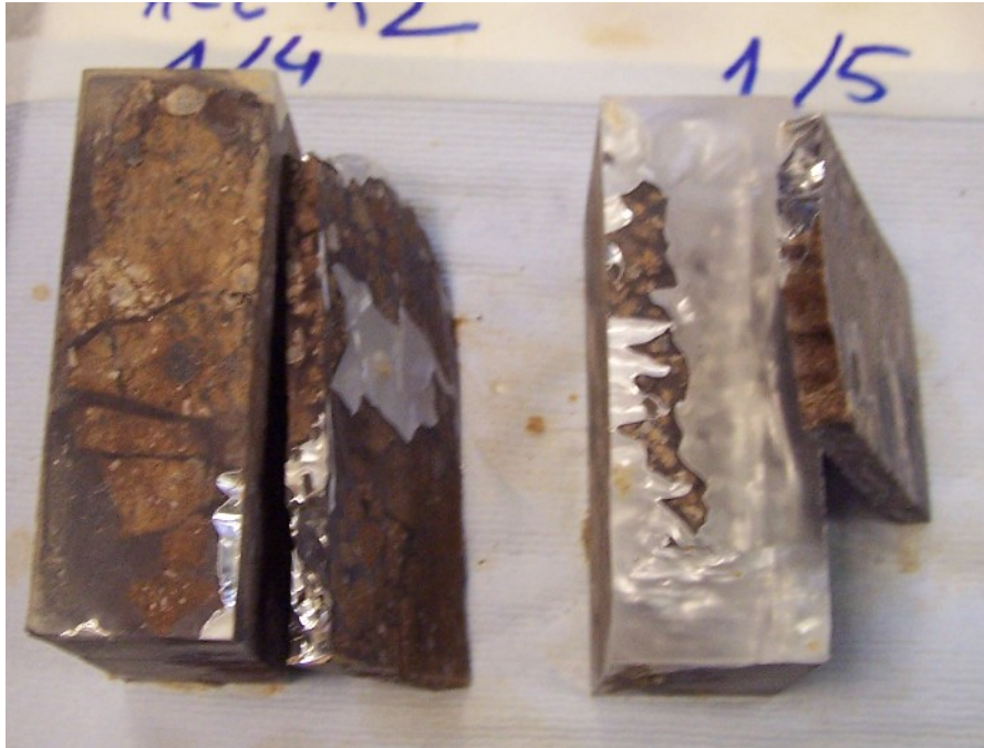
Figure 13: Cut blocks with a notch to indicate top of sample
