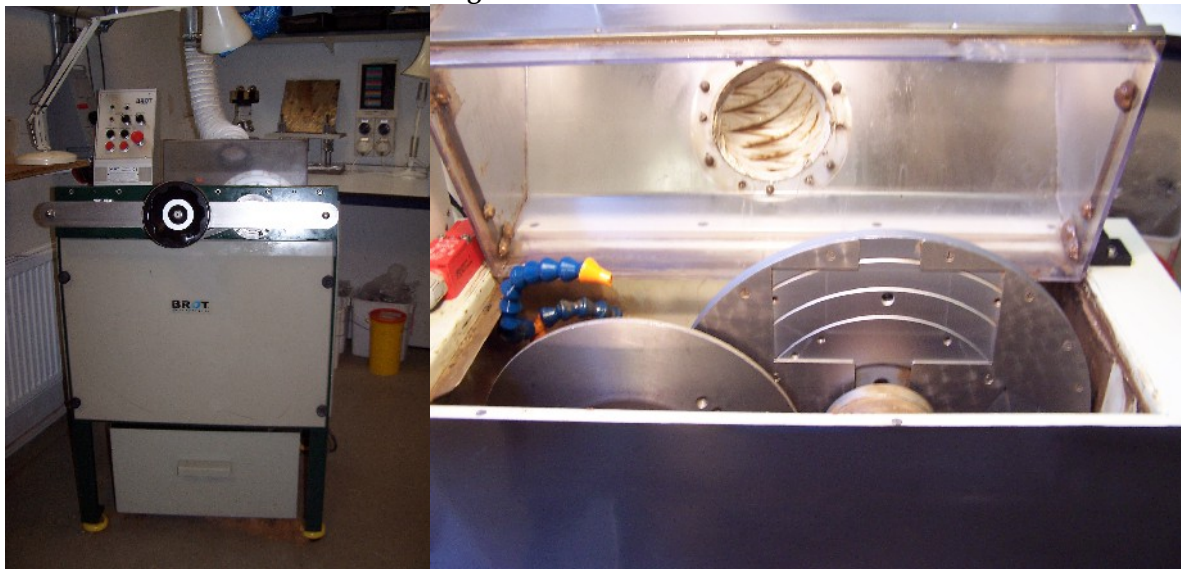
Figure 16: The Brot and its working area. Grinding wheel (l) and slide holder (r)
