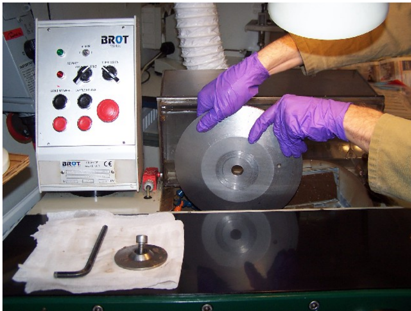
Figure 19: Changing the grinding wheel
